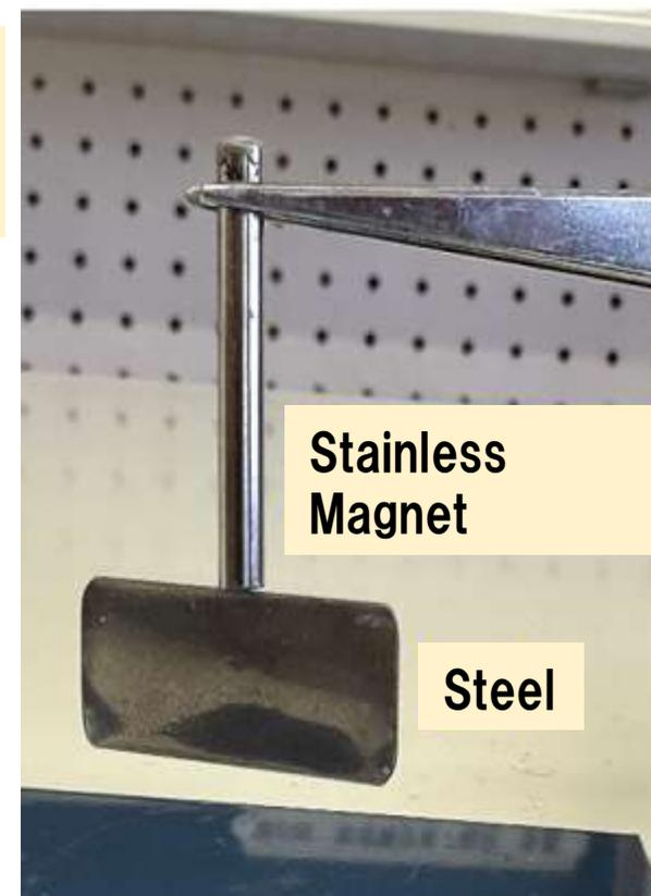
Steel is lifted up by a stainless magnet.
