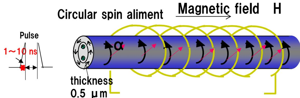
The wire has a **surface domains with circular spins**. When external magnetic field is applied to the wire along axis direction, spins tilt toward the axis direction.
