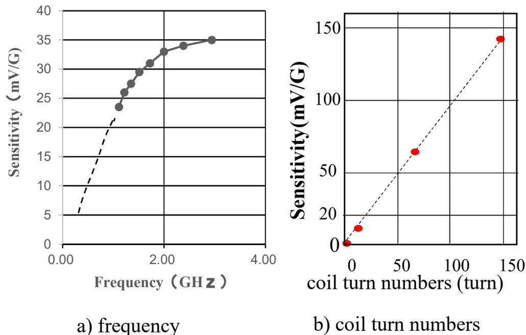
Fig. 7 Effect of frequency, coil turn numbers and wire permeability on Sensitivity
