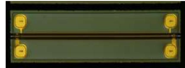
Wire terminal    Wire    Coil terminal
