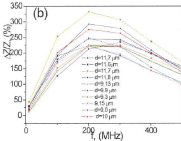
Figure 6. Frequency dependence of  $\text{Co}_{0.66.87}\text{Fe}_{0.3.66}\text{C}_{0.0.98}\text{Si}_{11.47}\text{B}_{13.36}\text{Mo}_{1.52}$  microwires with different metallic nucleus diameters
